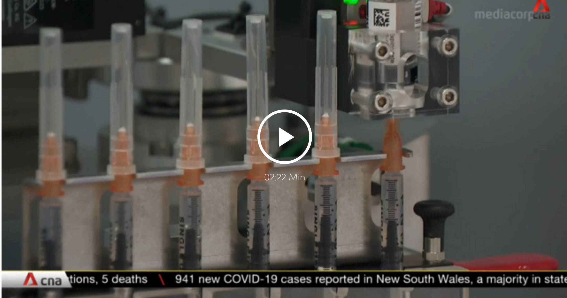
An automated vaccine extractor has been deployed at several COVID-19 vaccination centres, replacing the manual step of filling syringes with liquid doses. Sherlyn Seah reports.
