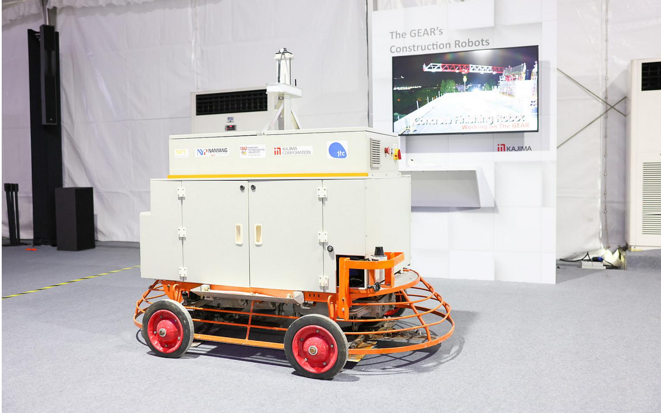
Kajima's concrete finishing robot can reduce labour costs by up to 30 per cent. PHOTO: KAJIMA DEVELOPMENT
